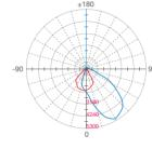
note : photometric result tested based on 11000lm MH 150W double ended tube
