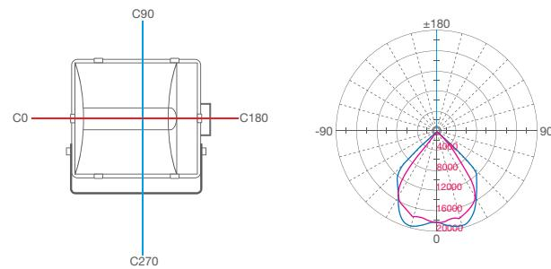
note : photometric result tested based on 180000lm MH 2000W clear tube
